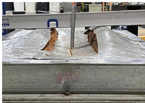
Deformation of granular material observed in the extra-large wheel tracking device
