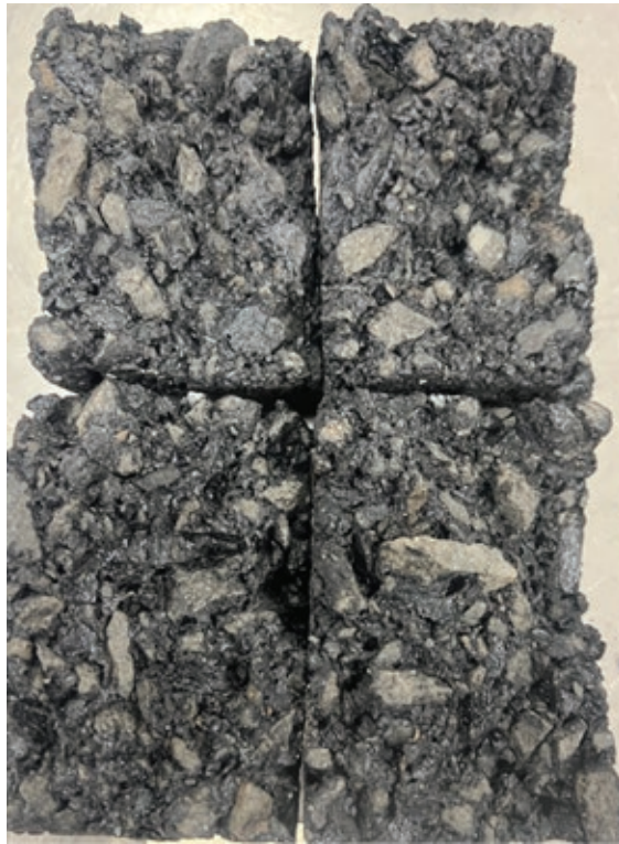
Asphalt stripping observed during the tensile strength ratio test
