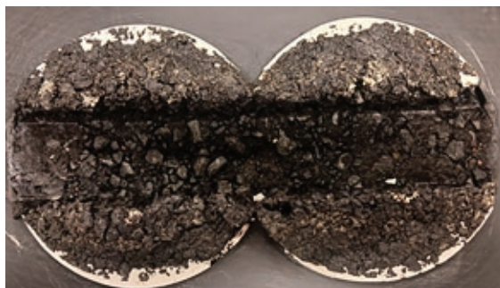
Asphalt stripping observed during the Hamburg wheel tracking test
