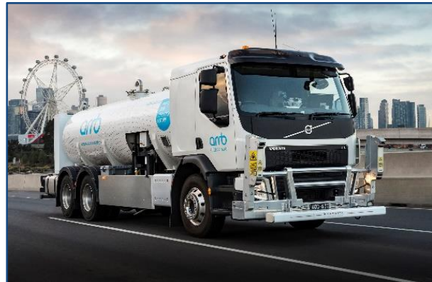
Figure 1.1: ARRB's skid resistance testing vehicle, iSSAVe
