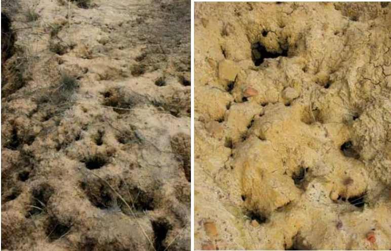
Figure 3.4: Example of pitting and pocketing of subsoil
