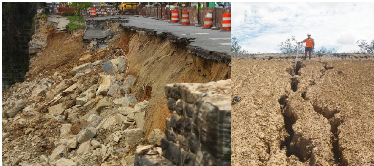
Figure 2.11: Example photos of dispersive soils
