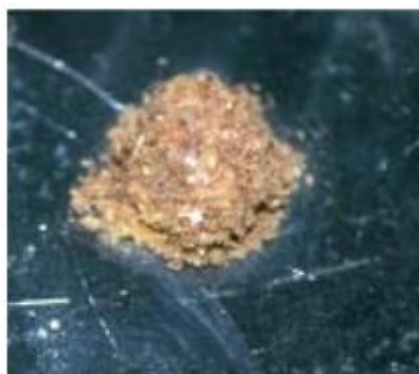
a. Soil lump has collapsed around the edges but remains mainly intact
