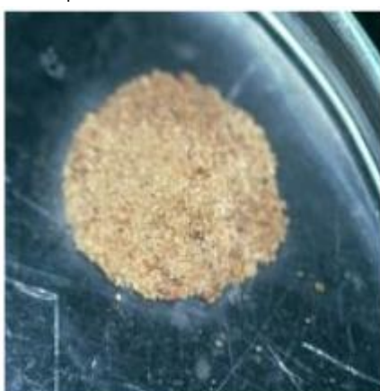
d. Soil lump has collapsed in single grains
