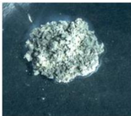
b. Soil lump has collapsed into angular pieces
