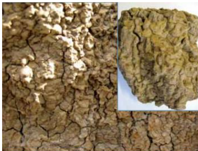
Figure 3.3: Example of dribble pattern on an exposed subsoil
