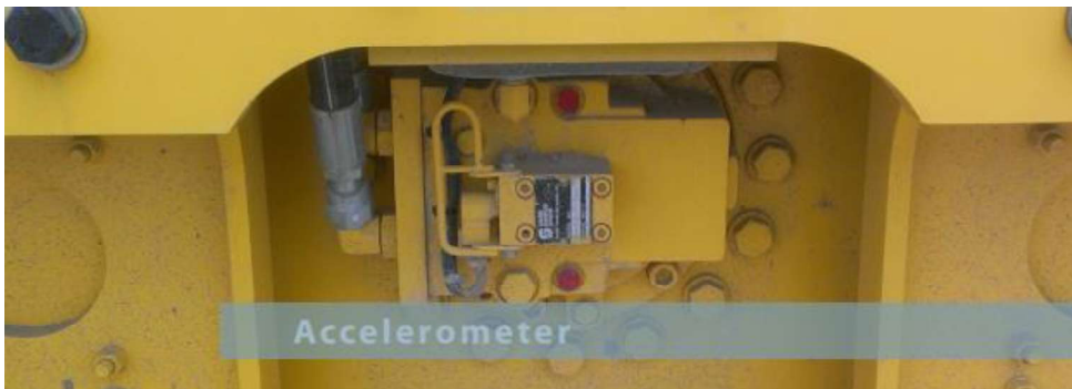
Figure 2.1: Accelerometer sensor mounted on the roller frame
