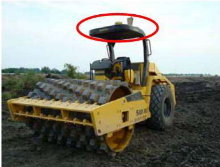
Figure 2.2: Real-time kinematic GPS receiver and antenna on a Sakai roller
