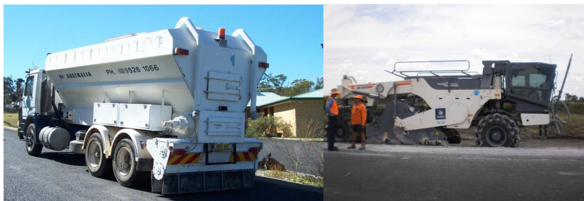
Figure 2.1: Modern powder binder spreader and recycler/reclaimer
