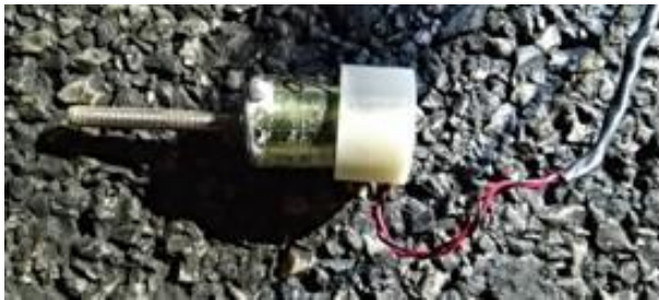
Figure 1.2: Geophone with protective cap installed
