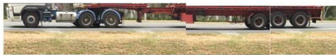
Figure 4.2: Example of an unladen three-axle group semi-trailer on Deception Bay Road
