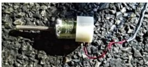
Figure 1.2 Geophone with protective cap installed
