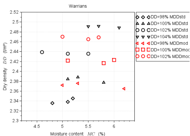
Figure 4.2: Dry density and moisture content conditions (Type 2.1 base material from Boral Warriars quarry)
