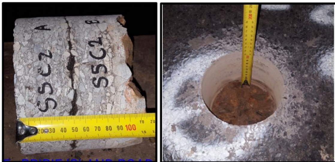
Figure 3.2 Asphalt core sample photos of Site 5 – Bribie Island Road 2
