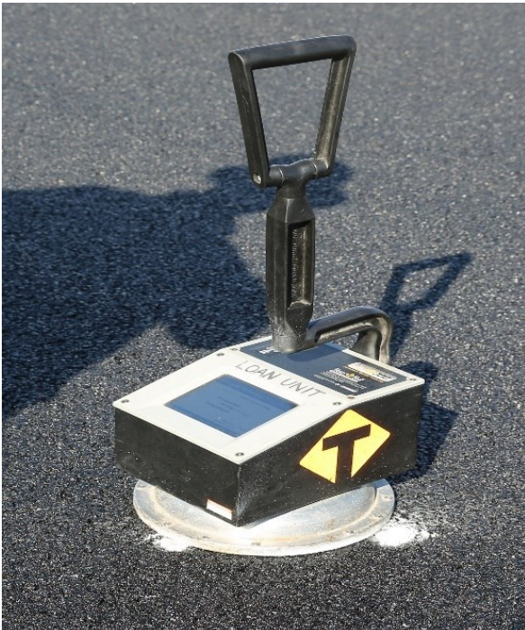
Figure 4.8: PQI taking density measurements
