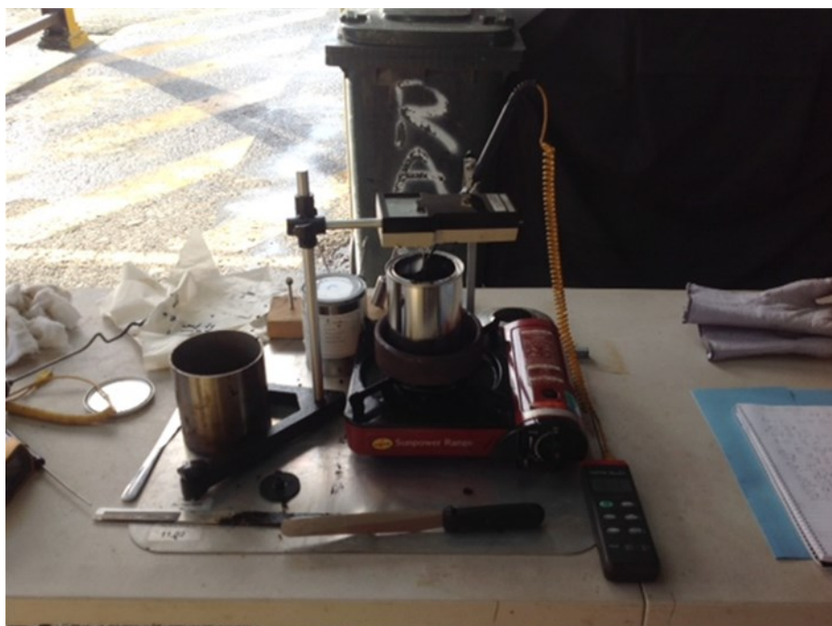
Figure 4.5: Hand-held viscometer used for testing
