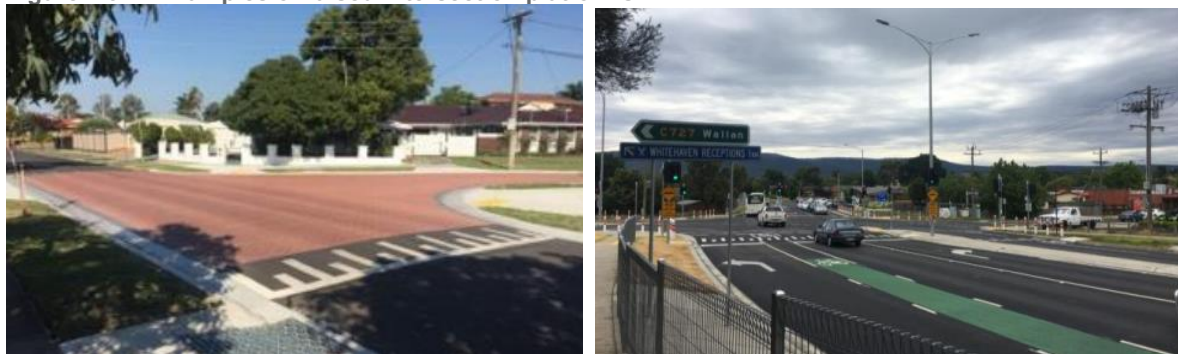
Figure 2.3 Examples of raised intersection platforms
