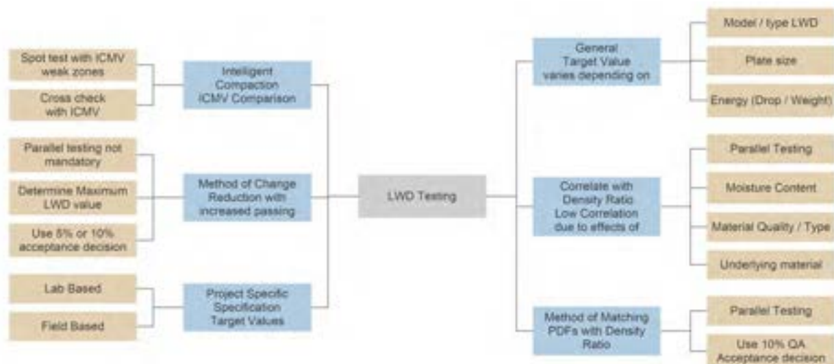
Figure 4-1 Various approaches to apply LWD testing
