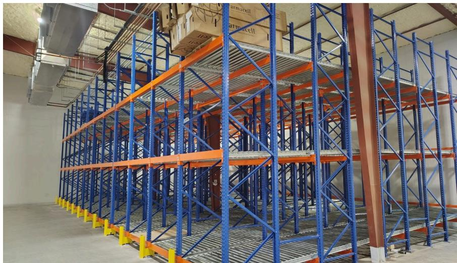
Racking systems provide organized, high density storage for palletized product, field bins, packaging, and agricultural supplies. Engineered for strength and operational flexibility, these systems maximize vertical space and streamline warehouse, cold storage, and processing facility workflows.
