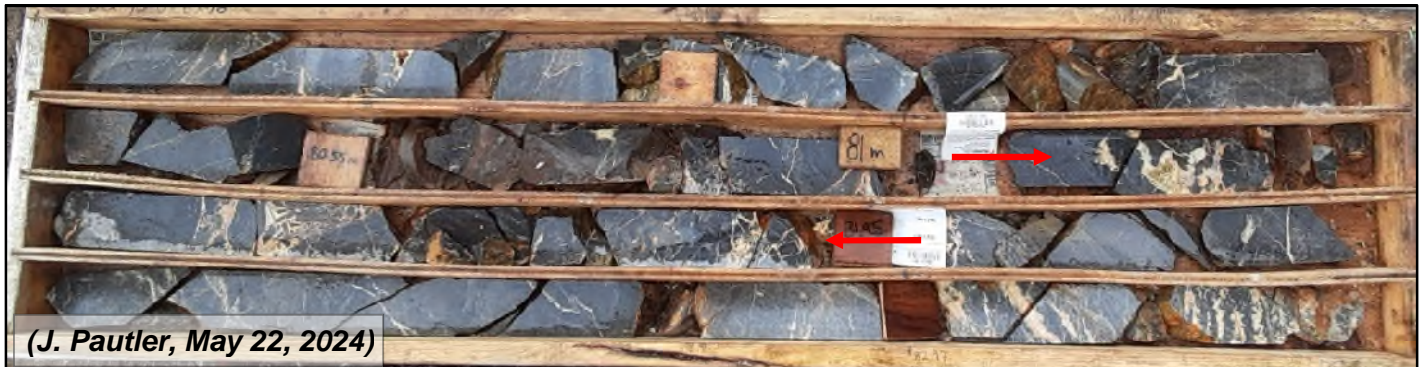
Photo 7: DDH D2-12-05, 49.3-49.3m Sample 1311702, dolomite breccia (resampled as E5532274)
