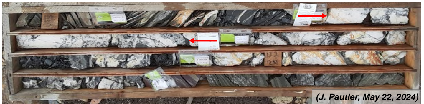
Photo 8: DDH J-21-015, 119.75-120.75m Sample 1311704, quartz-carbonate veins and breccias (resampled as C954781)
