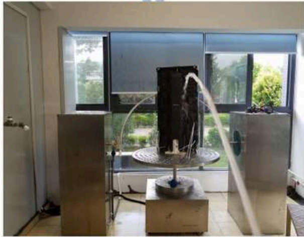
Fig.4 IPX5 testing (rear side)
