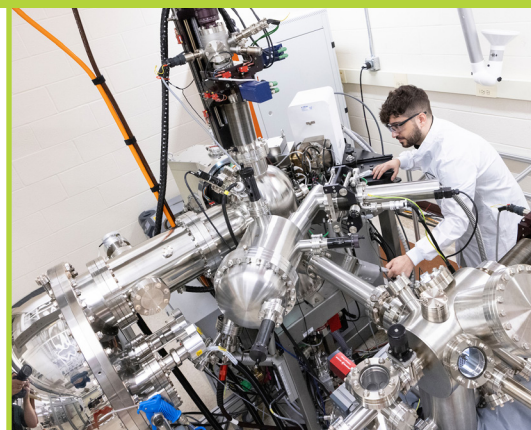
Above: The Analytical and Diagnostics Laboratory at Binghamton University, is home to a HArd X-ray PhotoElectron Spectroscopy (HAXPES) that's useful for electrode studies.
