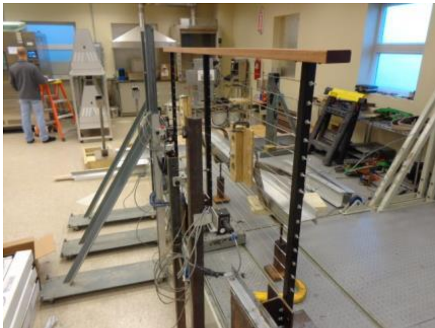
Photo No. 6 In-Fill Load Test - RailEasy™ Spectrum
