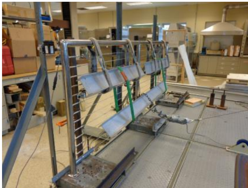
Photo No. 14 Uniform Load Test of Top Rail (Horizontal) - SunRail™ Nautilus
