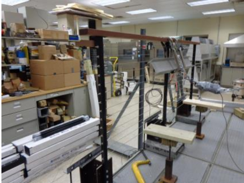
Photo No. 9 Concentrated Load Test at Top of Post Mount - RailEasy™ Spectrum
