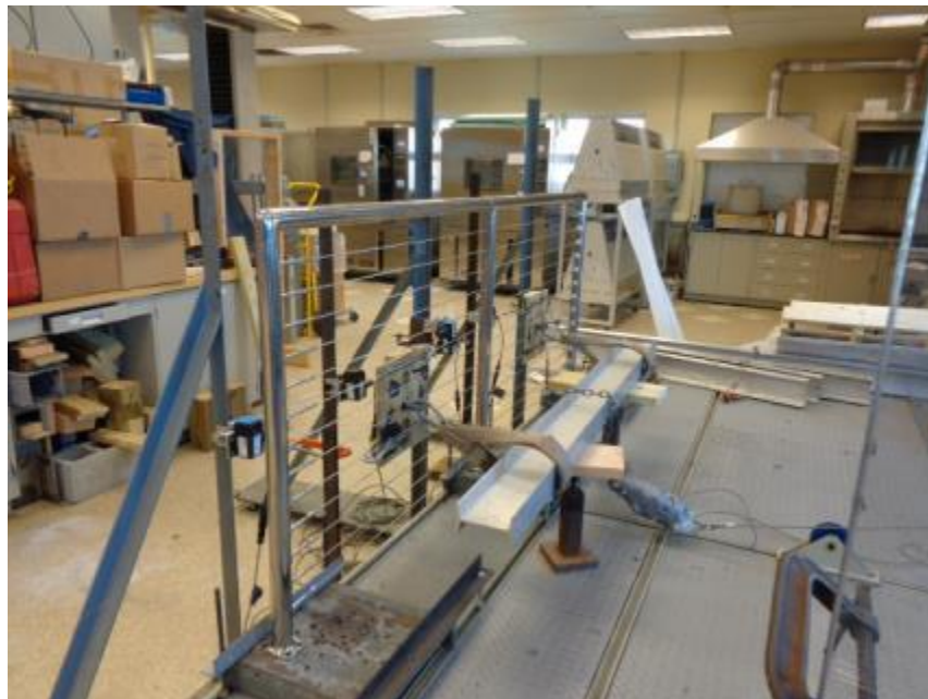
Photo No. 12 In-Fill Load Test - SunRail™ Nautilus
