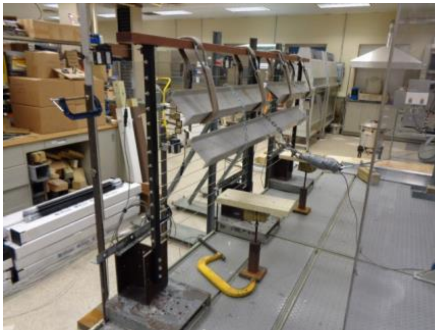
Photo No. 8 Uniform Load Test of Top Rail (Horizontal) - RailEasy™ Spectrum
