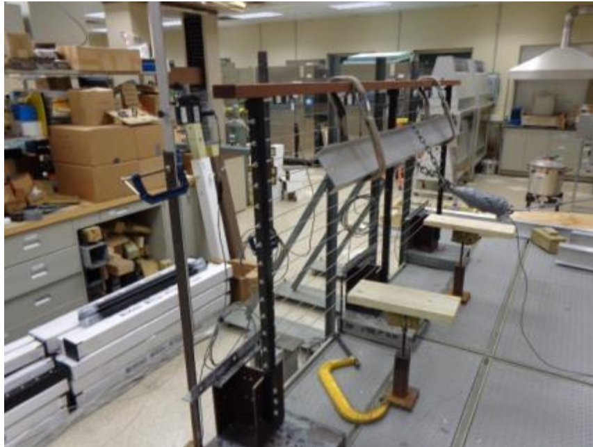
Photo No. 7 Concentrated Load Test at Mid-Span of Top Rail – RailEasy™ Spectrum
