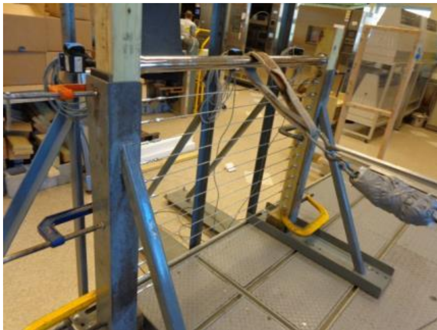
Photo No. 2 Concentrated Load Test at Mid-Span of Top Rail - RailEasy™ Nautilus
