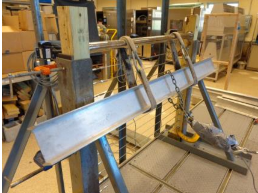
Photo No. 3 Uniform Load Test of Top Rail (Horizontal) - RailEasy™ Nautilus
