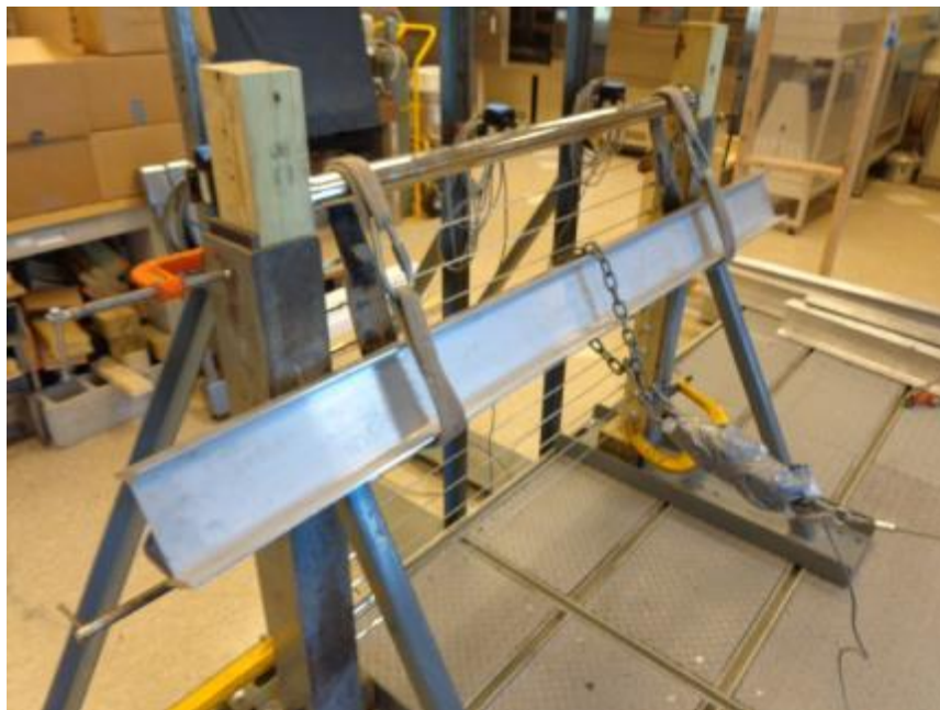
Photo No. 4 Concentrated Load Test at Ends of Top Rail (Brackets) - RailEasy™ Nautilus
