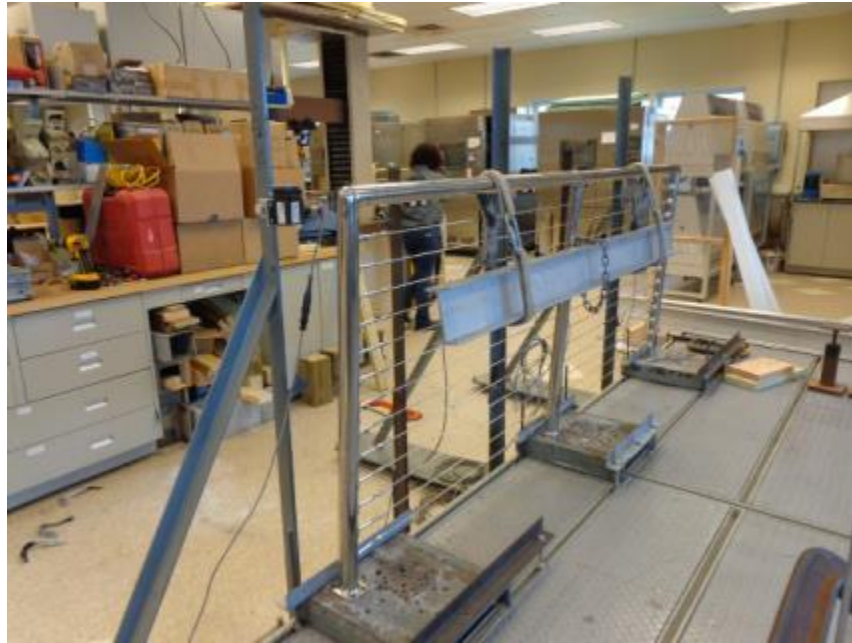
Photo No. 13 Concentrated Load Test at Mid-Span of Top Rail - SunRail™ Nautilus
