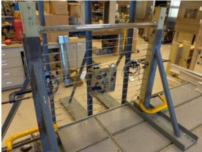
Photo No. 1 In-Fill Load Test - RailEasy™ Nautilus
