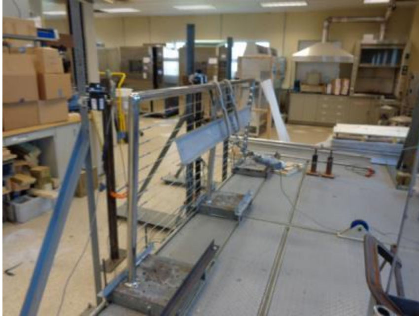
Photo No. 15 Concentrated Load Test at Top of Post Mount - SunRail™ Nautilus
