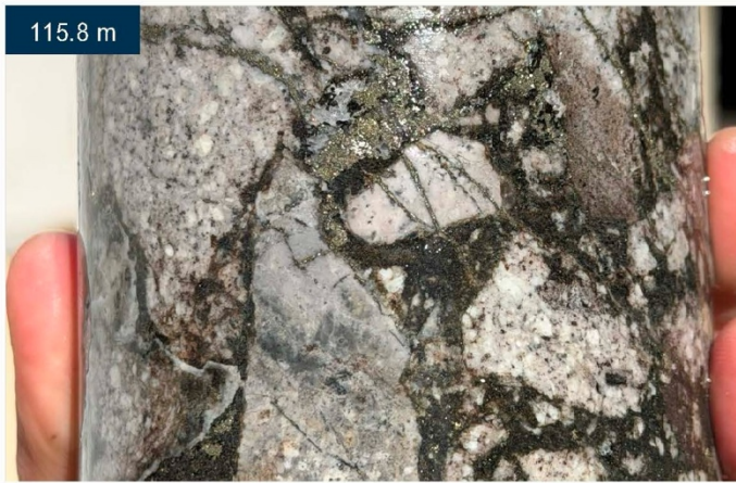
115.8 m Biotite–anhydrite altered breccia Magmatic hydrothermal breccia with matrix altered to biotite and anhydrite. Note pyrite and chalcopyrite. Assays from 115.0 m: 0.43% Cu · 0.29 g/t Au · 0.4 g/t Ag · 22.2 ppm Mo
