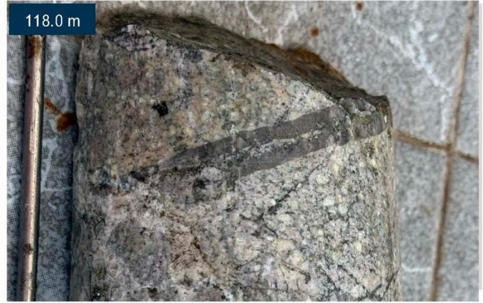
118.0 m Potassic-altered breccia with chalcopyrite Magmatic hydrothermal breccia with early potassic alteration partially replaced by silica–sericite alteration associated with chalcopyrite; note the early “B” family veinlet truncated at the fragment boundary. Assays from 118.0 m: 0.63% Cu · 0.88 g/t Au · 4.2 g/t Ag · 105 ppm Mo
