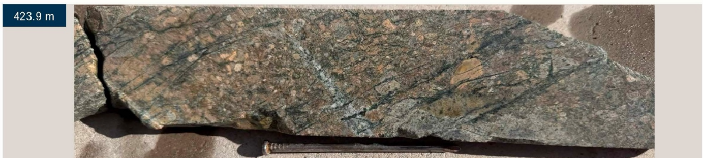
423.9 m Potassium feldspar replacement of phreatic breccia dike Fine-grained potassium feldspar replacement of phreatic breccia dike cutting across andesite wall rock; note the magnetite veinlets. The increasing intensity of potassic alteration with depth in FS_DD016 is a promising indicator of potential for a porphyry target at depth. Assays from 422.0–424.0 m: 0.04% Cu · 0.03 g/t Au · 0.26 g/t Ag · 8.6 ppm Mo
