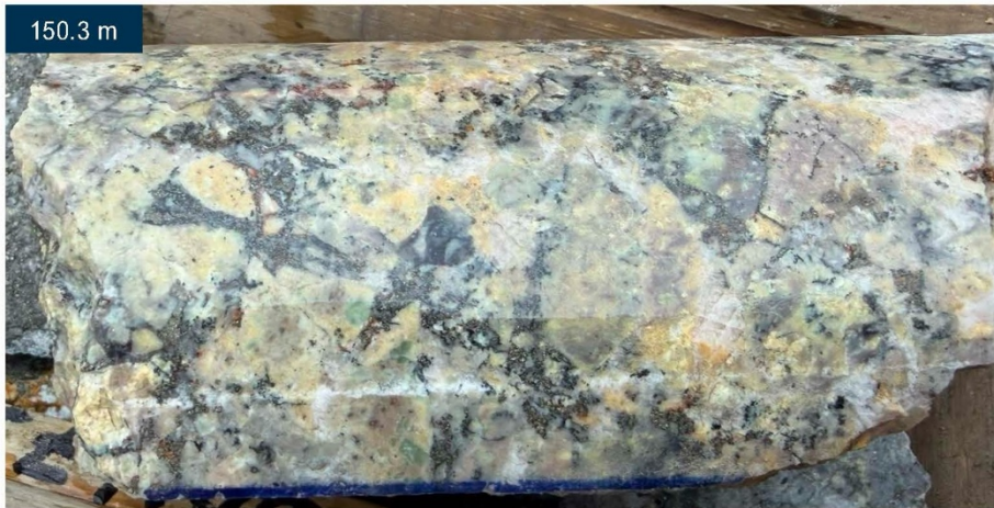
150.3 m Silicified breccia with epithermal sulfide overgrowths Silicified hydrothermal breccia with open space filled by pyrite and chalcopyrite, with epithermal overgrowths of dark copper-bearing sulfide minerals including probable covellite, digenite, bornite and enargite. Assays from 150.0 m: 1.5% Cu · 1.28 g/t Au · 3.3 g/t Ag · 417 ppm Mo
