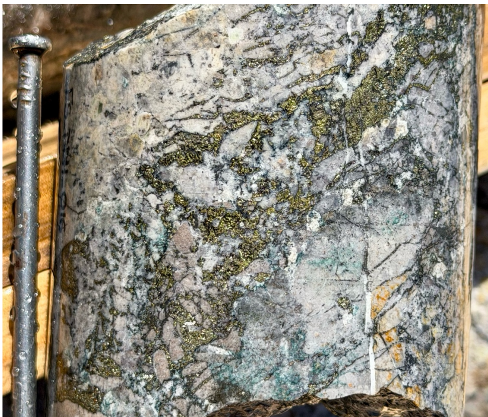
Figure 5: Core from 125.75m (FS DDH 016), 125-126m assays at 1.67% Cu, 1.62 g/t Au, 1.69 g/t Ag, 685 ppm Mo
