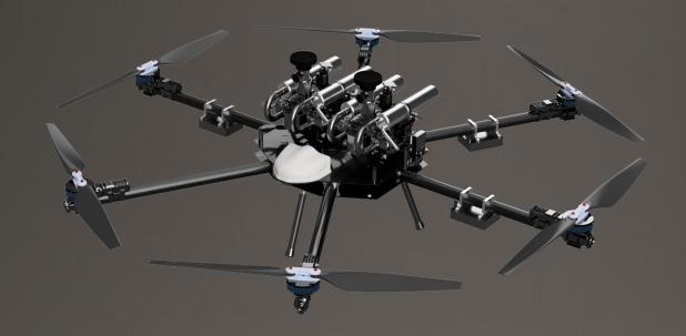
The Hecto Drone HD-606 is a state-of-the-art heavy lift hybrid multirotor aircraft designed for demanding aerial applications. Equipped with two generators and 6 motors, the HD-408 ensures robust performance and operational redundancy. Capable of lifting 50kg for 30 minutes or 25kg for 3 hours, this versatile aircraft is suitable for a wide range of applications.
