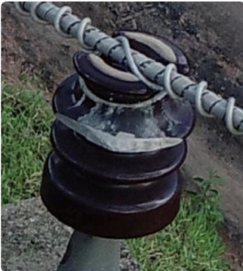
Broken ceramic pin insulator used for training an AI-model
