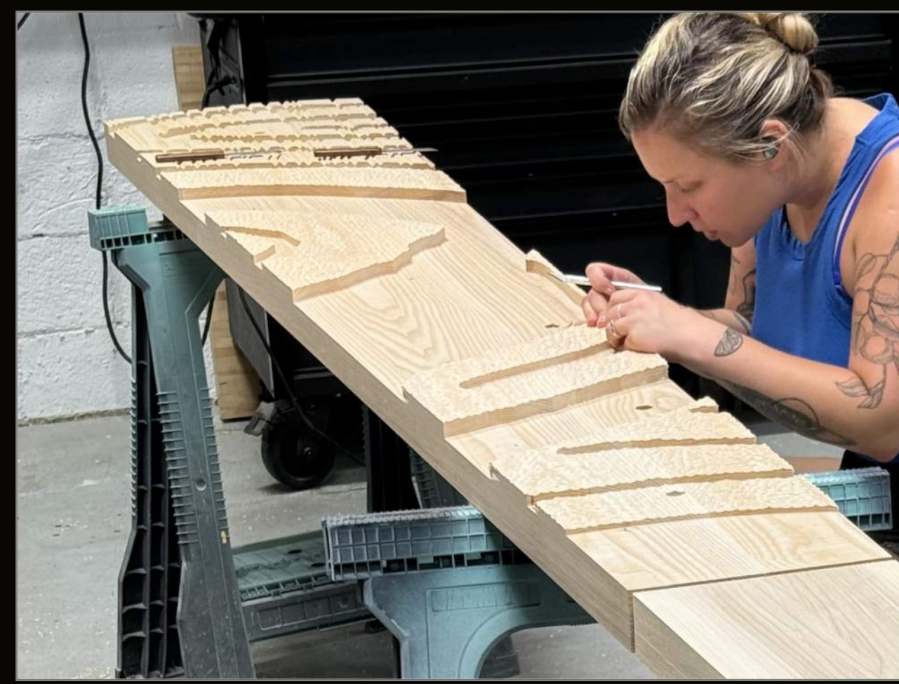
Center The full-scale visual mock-up panel receive patterning before raised wood elements are placed by hand into the recessed grooves shown here.
