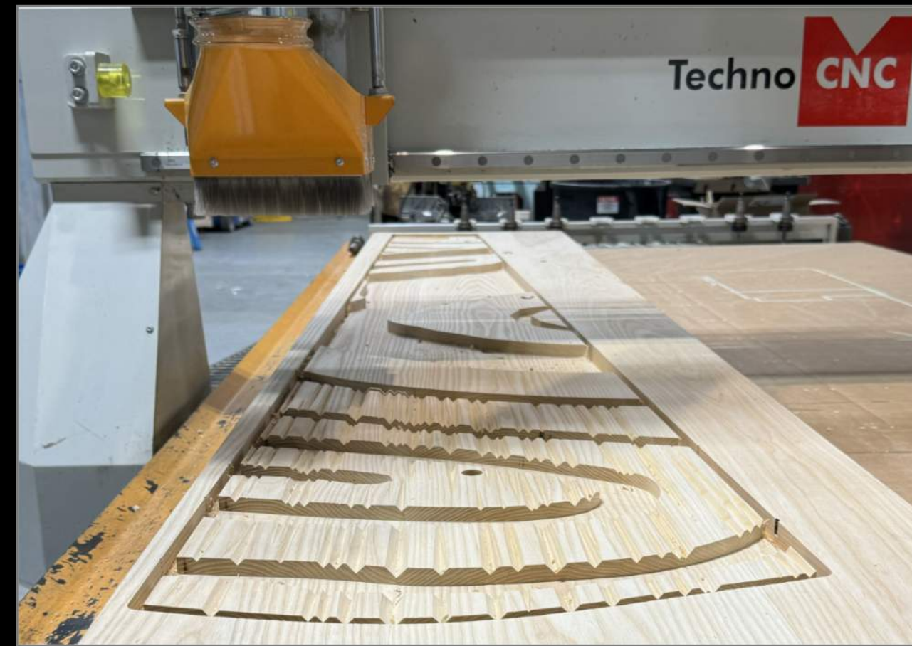
Center The full-scale visual mock-up panel receive patterning before raised wood elements are placed by hand into the recessed grooves shown here.
