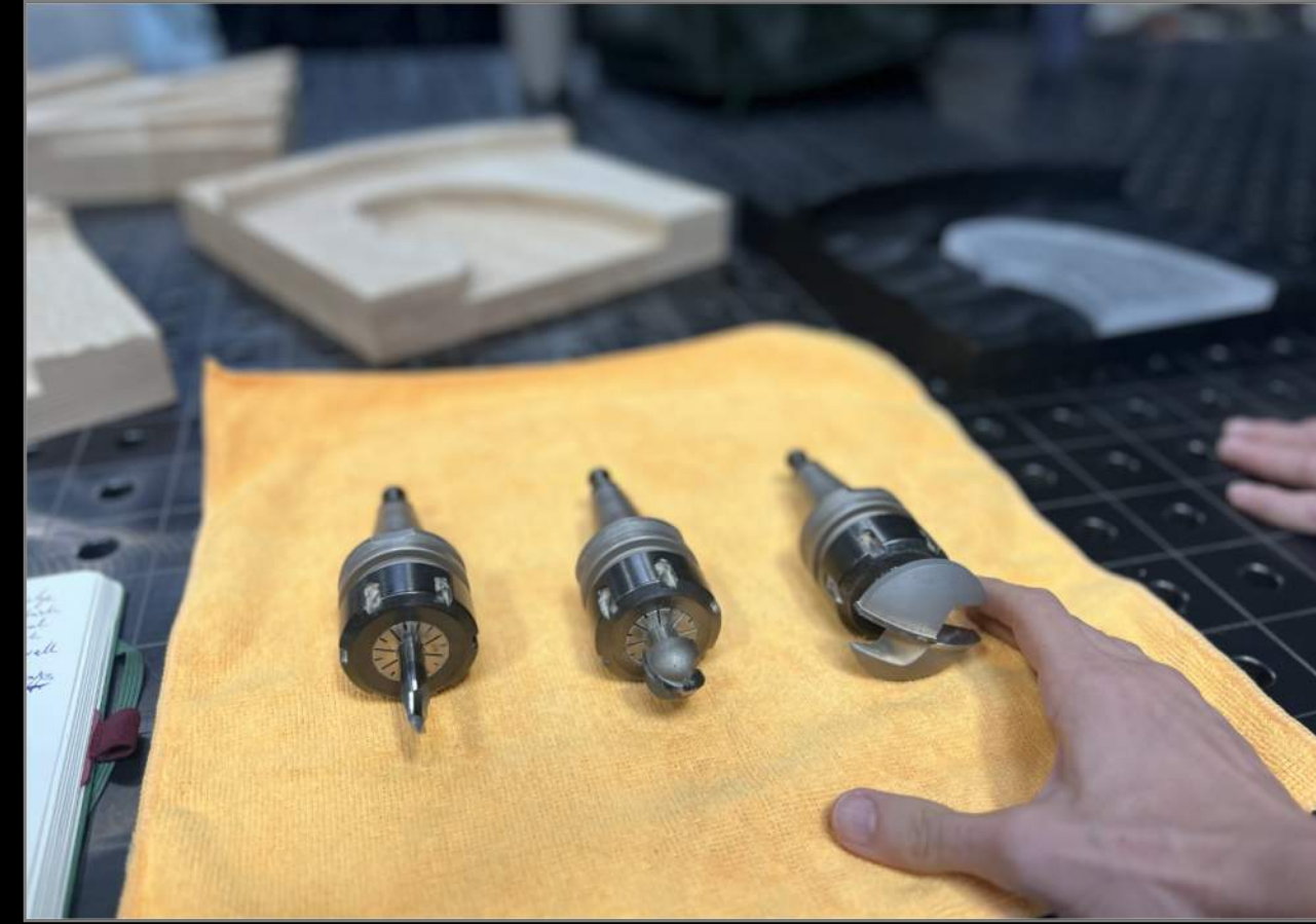
Top Three separate drill bits are utilized by the CNC machine to create many distinct wood patterns that were customized and parametrically designed so every inch of each 129 panels is unique.
