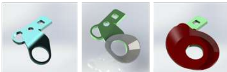
Figure 1. Brain Observatory Headframe and well. Isometric view of the custom headframe (manufactured from 1.6 mm (.063 inch) thick titanium 6Al-4V) and light-blocking wells for Scientifica (CENTER) and Mesoscope (RIGHT).
