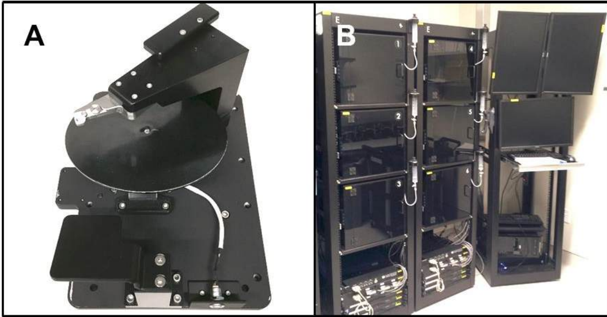
Figure 8. Behavior training platform. (A) Custom behavior stage equipped with a fixed-position headframe clamp and adjustable-height running wheel. The underside of the stage has a kinematic mount plate that mates to the floor of the behavior enclosure allowing reproducible placement of the stage in relationship to the LCD monitor (not shown). (B) Behavioral training clusters, allowing multiple mice to be habituated in parallel.
