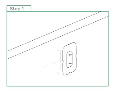
Align the U-Anchor 3000 series vertically, and install the U-Anchor attachment according to the instructions provided by Anchor Products.
