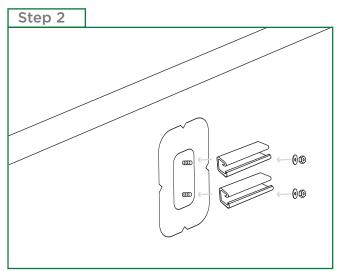
Attach the two pieces of channel strut horizontally. (One over the top bolt and the second over the bottom bolt.), the secure the channel strut using the provided stainless steel washer and nut.
