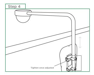
Position the height as needed and tighten the clamps.
