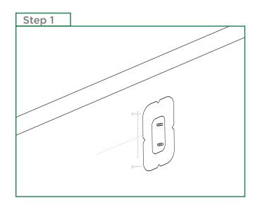
Align the U-Anchor on the parapet wall as per design requirements and attach the U-Anchor according to the install instructions provided by Anchor Products.
