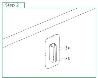
Attach the Three-sided Strut Bracket using the provided 3/8" Flat Washer and 3/8"-16 Flanged Nut. Tighten to 20 ft/lbs.
