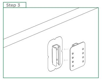
Secure the Attachment Plate to the Three-sided Strut Bracket using 3/8"-16 Spring Nuts and 3/8"-16 Stainless Steel Flathead Bolts.
