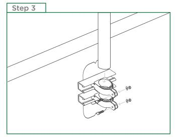
Secure the provided round pipe using properly sized pipe clamps.
