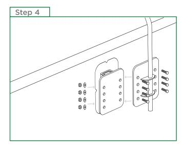
Secure the pre-assembled Camera Post and Plate to the previously attached plate using a minimum of 3/8" Flat Washers on each side of the plate and 3/8"-16 Nuts and 3/8"-16 Bolts.
