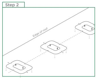
Align the U-Anchor as previously outlined. Use U-Anchor notches to mark your plot lines for the positions of the posts. Install the U-Anchor as per-product specific installation instructions.
