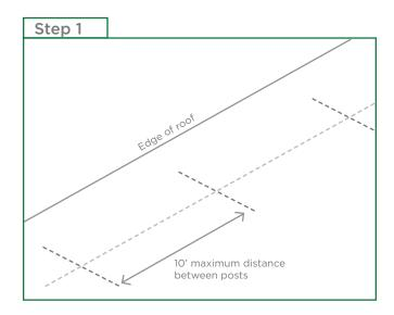
Determine location of the guardrail as per the engineered design. Convey the design to the roof surface using non-staining chalk to mark line.
