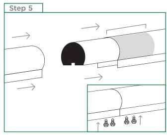
Insert the handrail and knee rail splice joints halfway into the respective rails. Fasten the splice joint with four (4) 3/4" fasteners per splice (Two (2) into each side of the splice.) Ensure that the handrails are tight together before fastening the final two screws.
