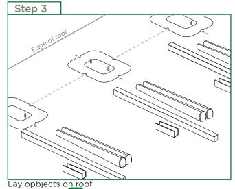
Layout the Handrails, Knee Rails and Post Components as per the project-specific design. Ensure splice joints will not be installed directly over the posts.
