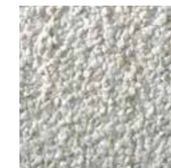
M: Medium [3-5 mm] Thickness: 8.0 ± 0.6 mm
