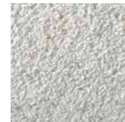
F: Fine [1-3 mm] Thickness: 6.5 ± 0.6 mm
