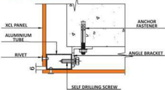
TYPICAL CORNER DETAIL TYPE 1 (PLAN VIEW)
