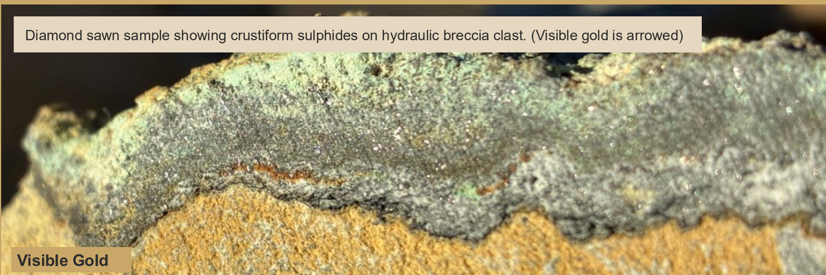
High-grade, colloform banded quartz-vein/breccia ore from the Night Reef
