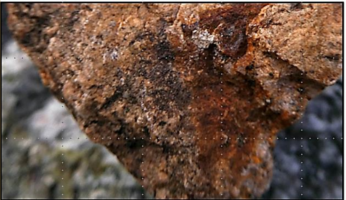
Banks Porphyry sample, showing fresh sulphides, thin veinlets, and high density of sulphidic fractures. Float rock assays up to 0.27% copper are associated with extensive detrital gold dispersion downstream.
