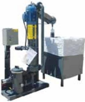
**GRS – Garnet Removal System** – automatically and continuously removes the used spent abrasive from the main catcher tank without downtime associated with cleanout. The GRS includes a sweeper package inside the tank which pumps the abrasive out of the tank into a settlement tank liner bag which is easily removed to a waste dumpster.
