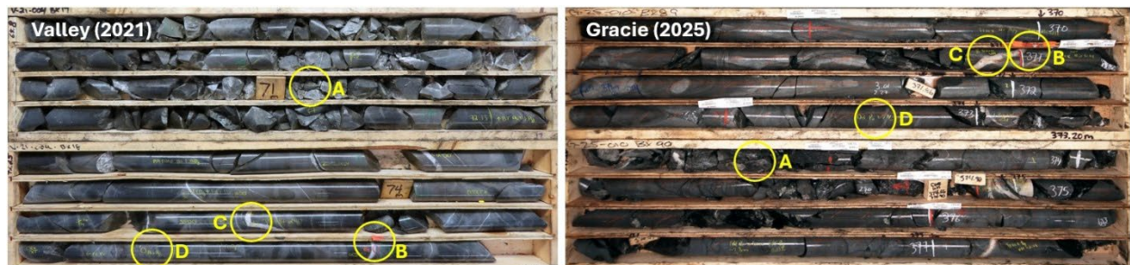
Figure 3 – An early “near miss” from Valley, V-21-004 (left) alongside core from G-25-010 from Gracie (right). V-21-004, the fourth hole drilled at Valley, intersected silicified sedimentary rocks with low quartz vein densities along a fault corridor, returning 0.77 g/t Au over 93.8 m roughly 50 m from the edge of the well-mineralized Valley intrusion. G-25-010, drilled last season at Gracie, intersected similar alteration and mineralization associated with a fault zone, returning 0.32 g/t Au over 53.5 m at an unknown distance from an intrusion. Similarities include: (A) Fault zone associated with alteration; (B) visible gold in quartz veins associated with bismuth and tellurium; (C) mineralized, centimeter-scale veins with irregular geometries; (D) disseminated pyrrhotite in silicified, fine-grained siliciclastic sedimentary rocks.
