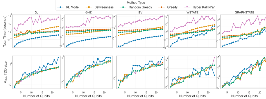
Figure 2: Performance comparison of the RL-based model and baselines across all benchmark families (log scales). The RL model consistently achieves lower contraction time, while the peak TDD size is less stable but overall similar.
