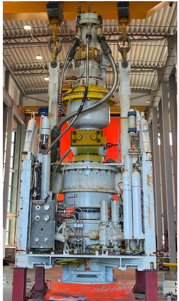
18-5M SGV shown configured with 10ksi top and bottom connections and illustratively installed in an LMRP.
