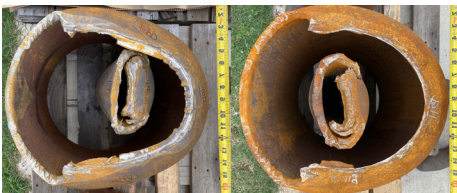
18" OD Casing, P110 6-5/8" OD Inner String, V150 Combined 167ppf
