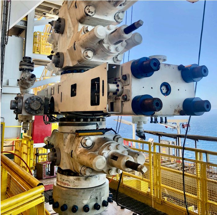
Shown Left: K-BOS added to a BOP stack as a replacement for the drilling cross flow spool.
