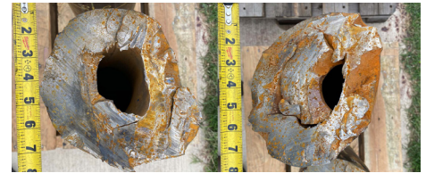
6.9" OD Slip Proof Landing String, V150 Side Load & Compression
