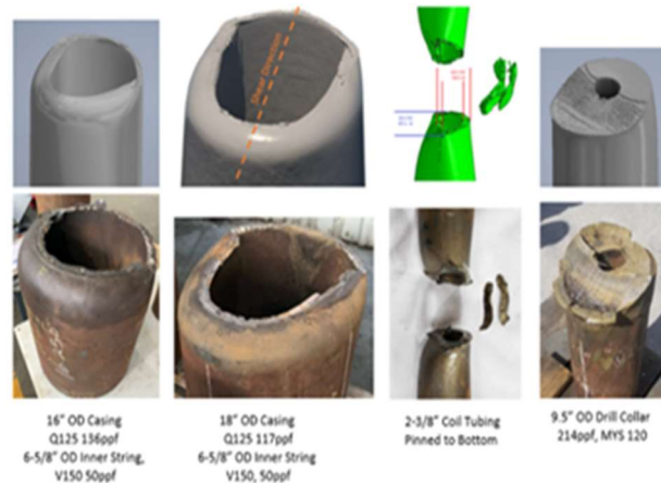
Figure 2- K-BOS shear modelling and shear samples
