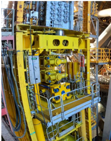
Figure 1- K-BOS Subsea BOP retrofit
