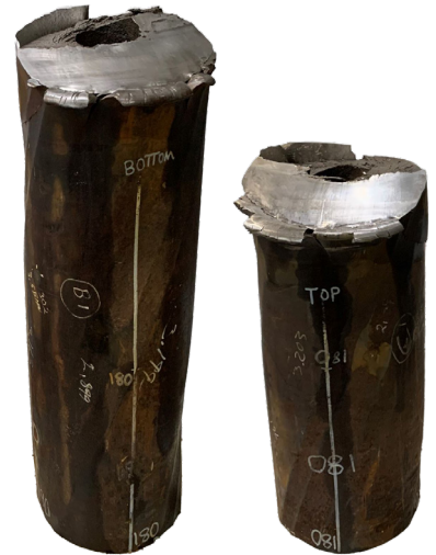
18-15M K-BOS shear test results on a 9.5" OD 120ksi MYS 214# Spiral Drill Collar
