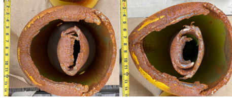
16" OD HP Casing, Q125 6-5/8" OD Inner String, V150 Combined 186ppf
