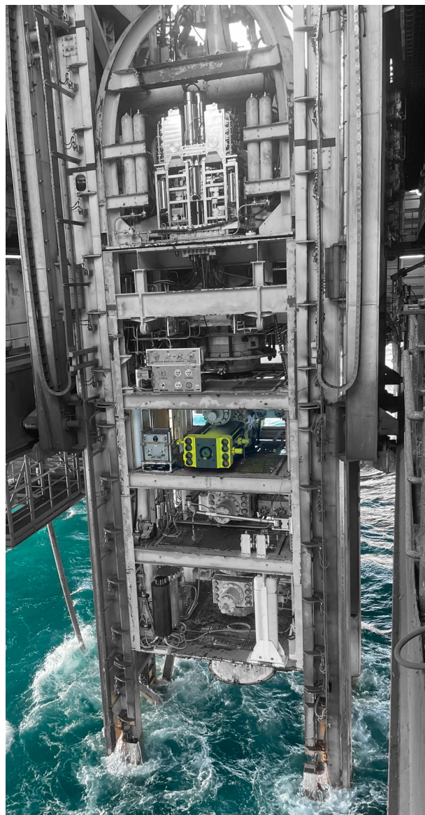
18-15M K-BOS retrofit installed in HMH / Hydril Compact BOP stack
