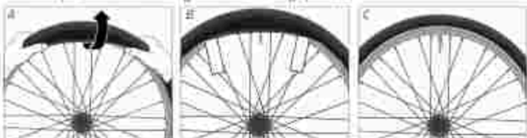
Illustr. Fitting clincher or folding tyres (CI)
