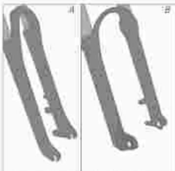
Illustr. Open (A) and closed (B) fork ends (leverless)
