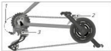
Illustr.: Components of a derailleur shifting system (example)
