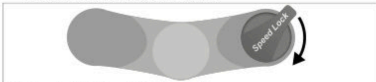
Illustr.: Suspension fork lockout control (top view, example).
