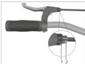
Illustr.: Lock nut and knurled screw position (example)
