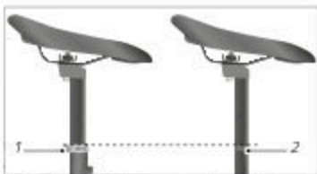
Illustr.: Seat post minimum insertion depth (example)
