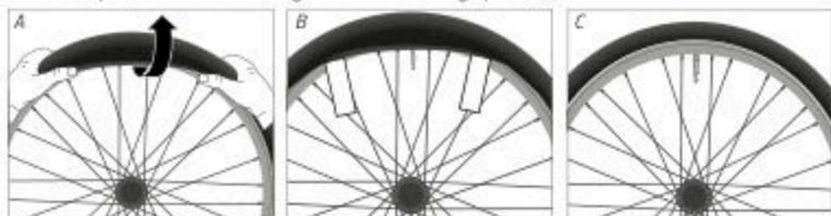
Illustr.: Fitting clincher or folding tyres (example)
