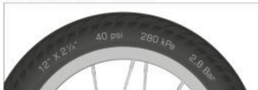
Illustr.: Tyre with tyre size specification (example)
