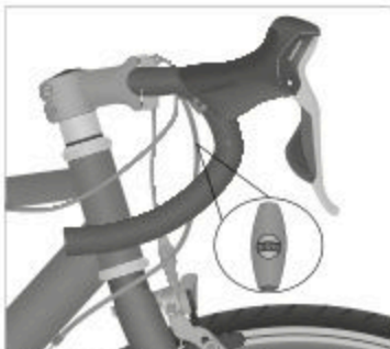
Illustr.: Adjusting the derailleur shifting system (example) Adjustment screw with wheel for adjusting the cable tension
