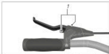
Illustr.: Adjustment screw position (example)
