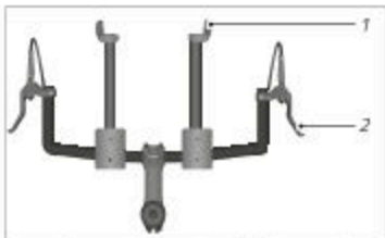
Illustr.: Distance between the shift levers and brake levers on aero handlebars (example)
