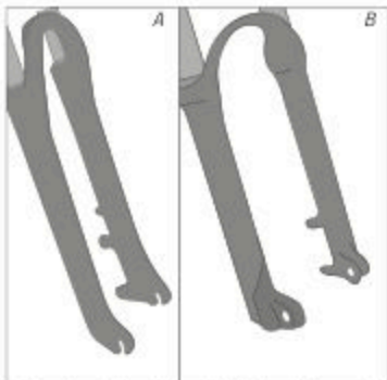
Illustr: Open (A) and closed (B) fork ends (example)
