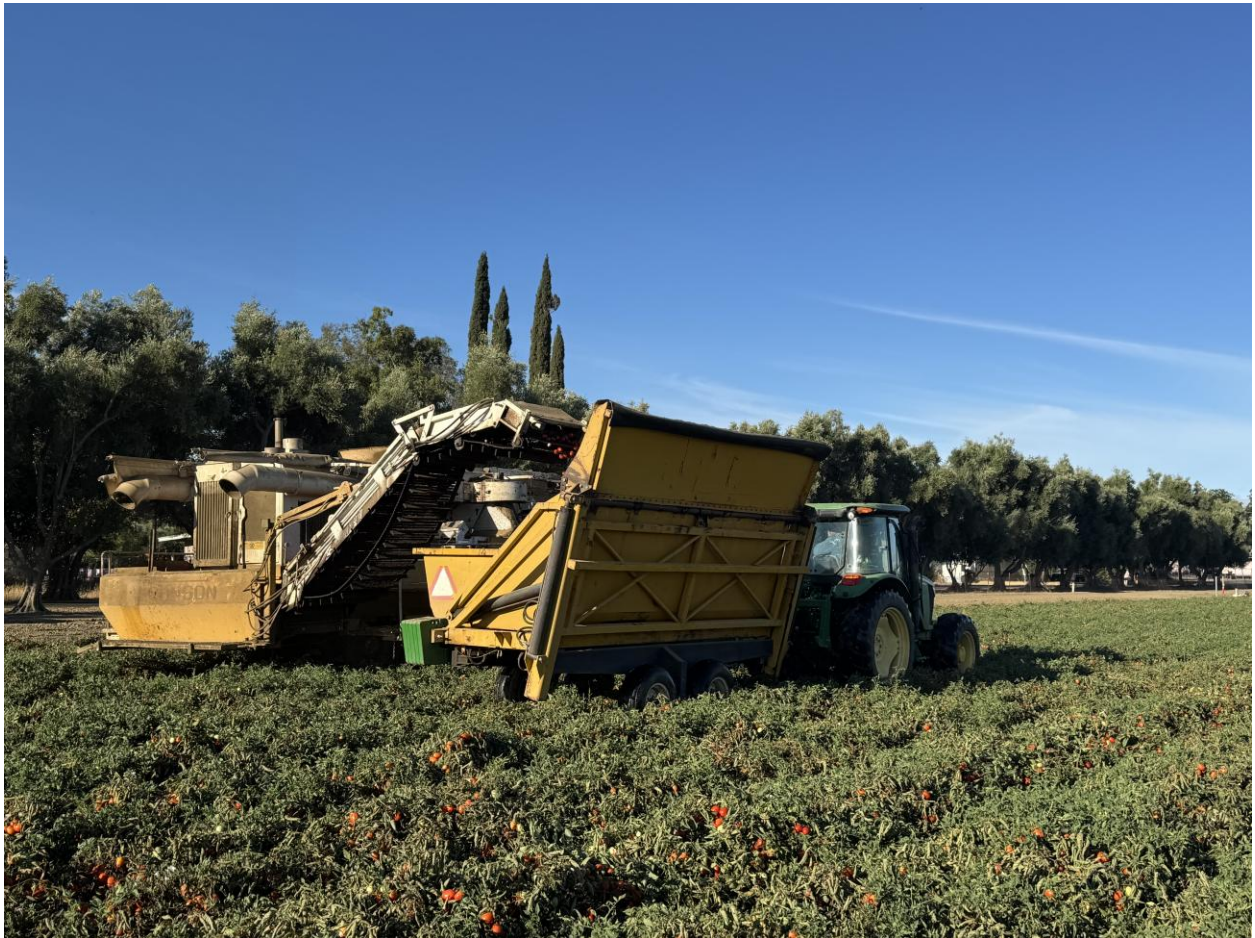
Figure. 2. Commercial mechanical harvest of processing tomatoes using a Johnson tomato harvester. The machine cuts the vines and conveys fruit onto an onboard sorting and cleaning system before transferring marketable tomatoes into a tractor-pulled collection trailer.
