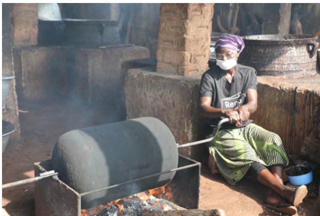
Figure 3: Improved roaster installed at GUBDANDA Shea Butter Processing Centre
