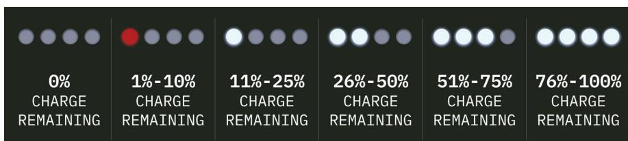
When the battery is powering the Sidekick, the red LED will slowly blink to inform you of low charge when there is about 5 minutes left before the battery shuts off. Otherwise, all LEDs will display solid.
