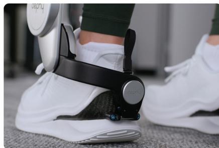
Hold the Sidekick vertically at the heel of your shoe. Rest the hooked connector against the magnetic bar on the shoe cleat, then rock the device forward until you hear an audible click. This ensures the connection is secure.
