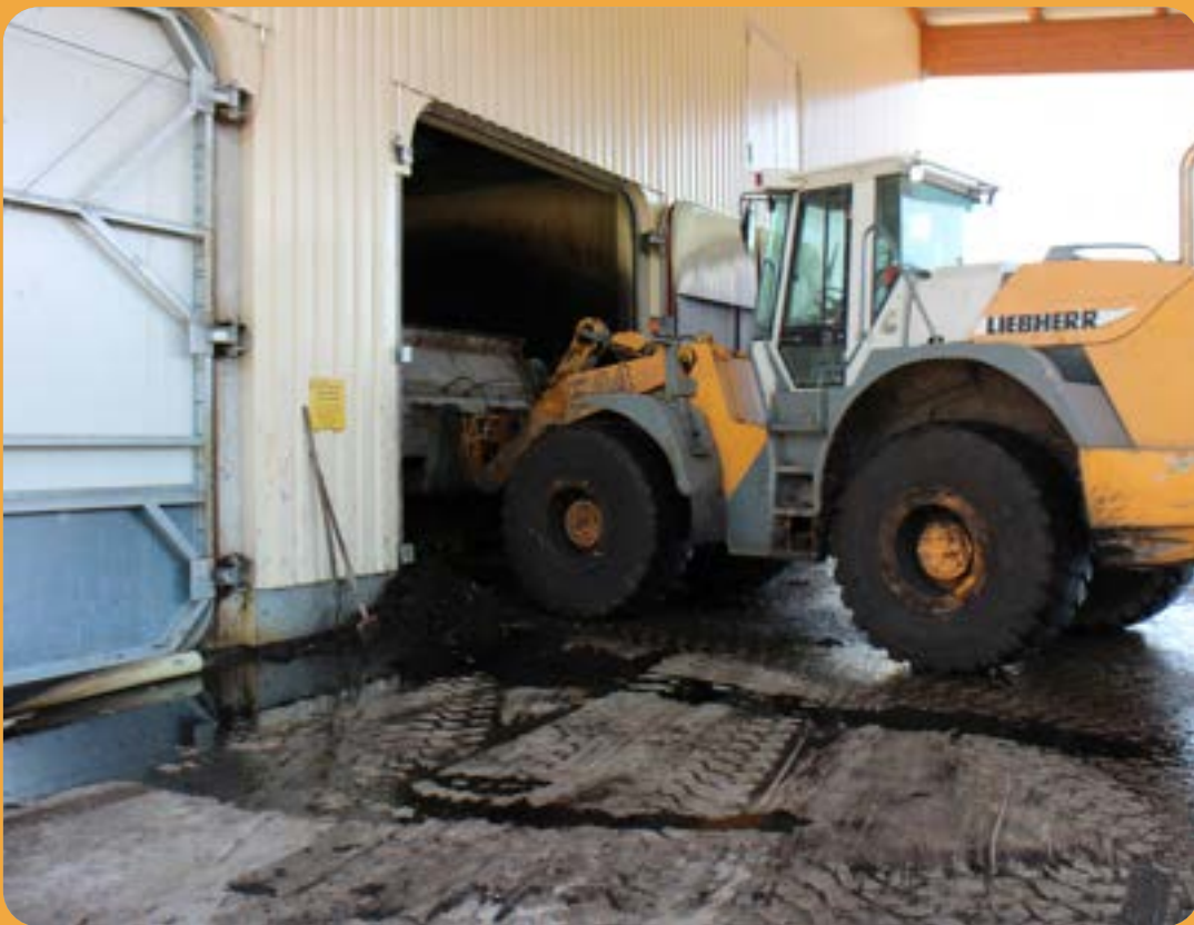
FIGURE 5: FILLING SOLID ORGANIC MATERIAL INTO A TYPICAL BATCH SYSTEM AD FACILITY USING A LOADER AT ONE UNIT IN THE ARRAY OF CHAMBERS
