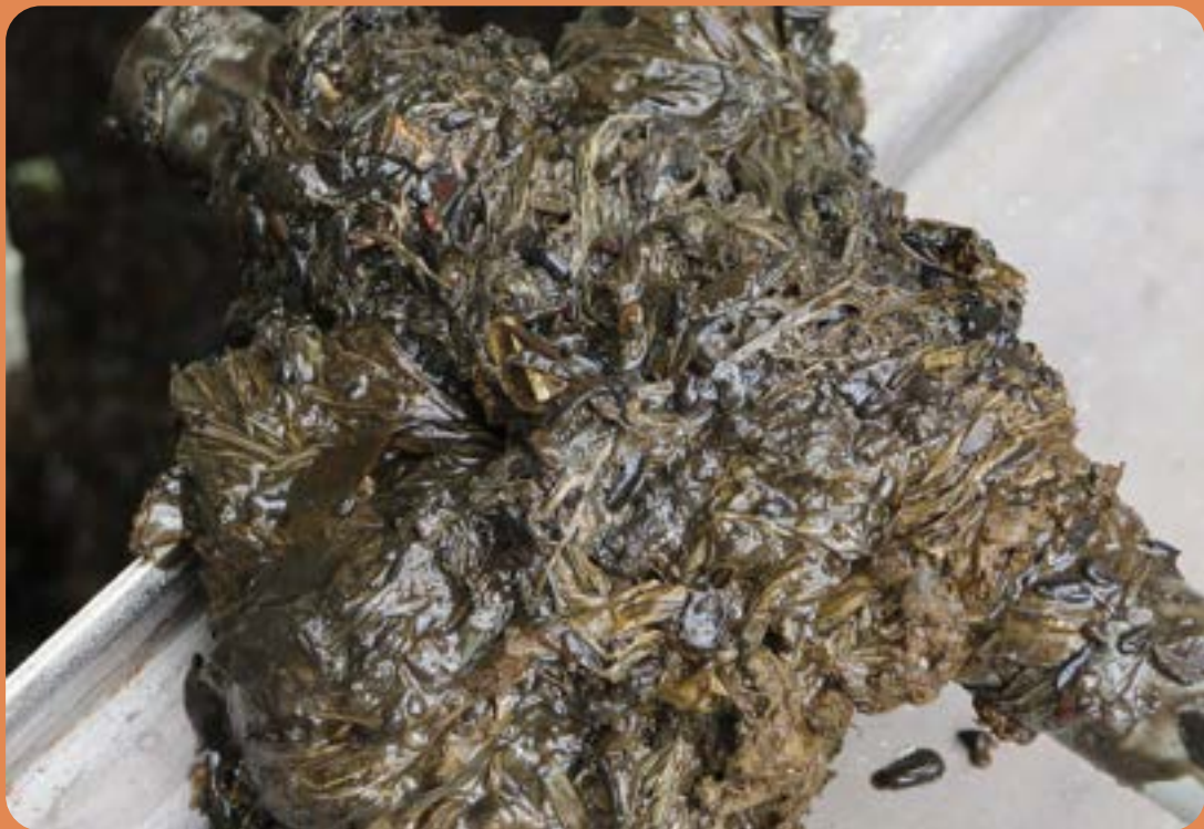
FIGURE 9: CLOSE UP OF COALESCED COMPOSTABLE PLASTIC FORMING A FLOATING LAYER IN A MESOPHILIC WET DIGESTER
