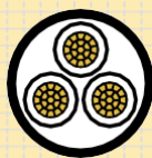
Construction of 3 core cable
