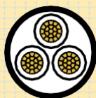
Construction of 3 core cable
