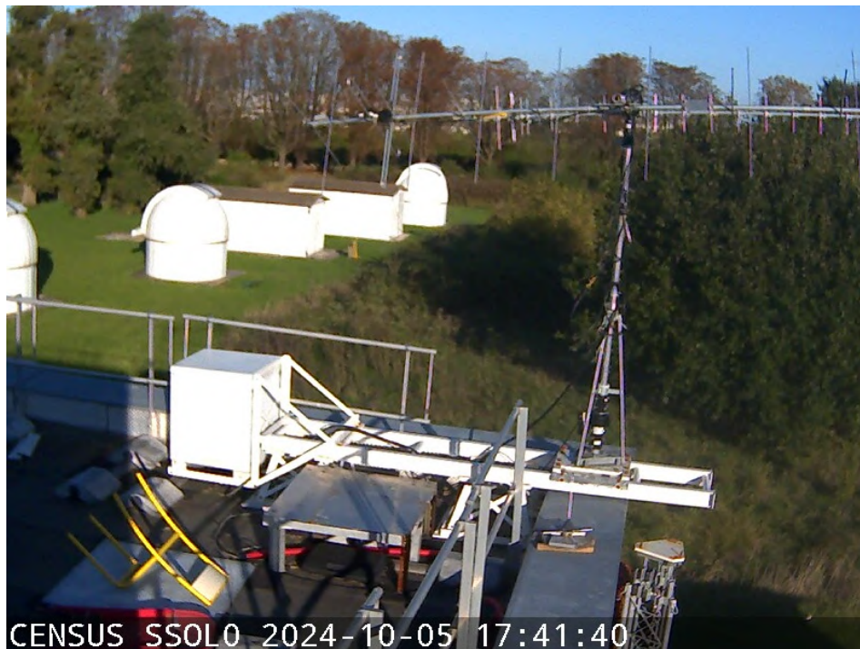
Figure 6: SSOL in Meudon (from webcam, optical distortions). Here the pylon spire structure is detached from the pulley system.
