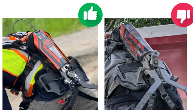
Examples of a clean (left) and soiled (right) exoskeletons
