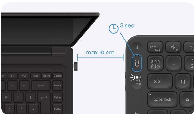
**Step 4:** Bring the keyboard's upper-left corner within 10 cm of the dongle
