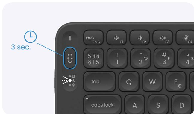
Press and hold the QuickSwitch button for 3 seconds
