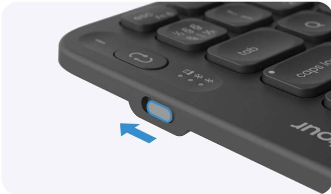
**Step 1:** Turn on the keyboard using the slider on the left side
