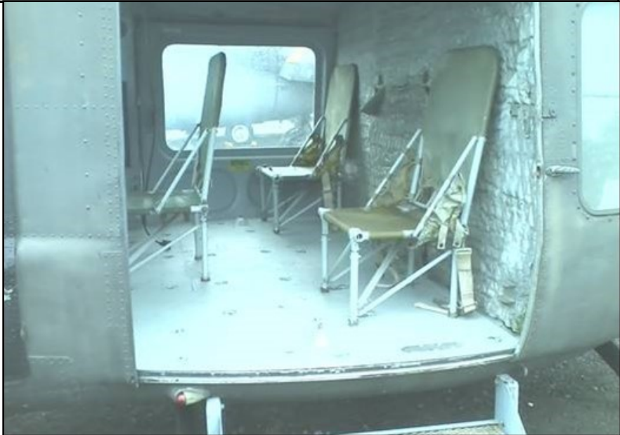
Restored seats in the Huey passenger cabin
