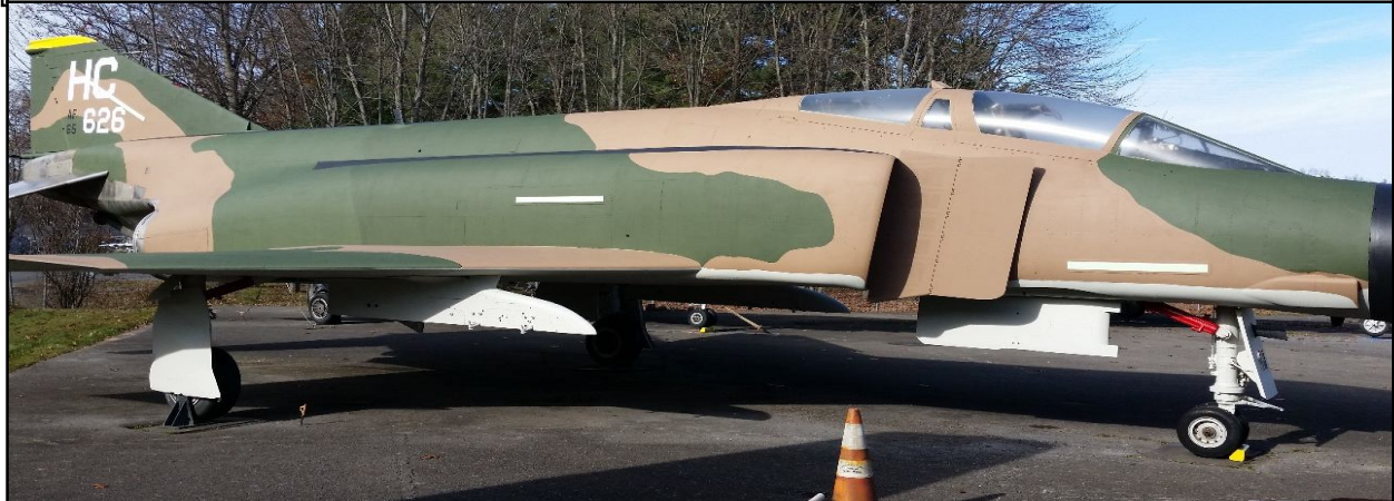
Glow Bars on Tail, Fuselage, and Wingtips were used at Night to facilitate Close Formation Flight
