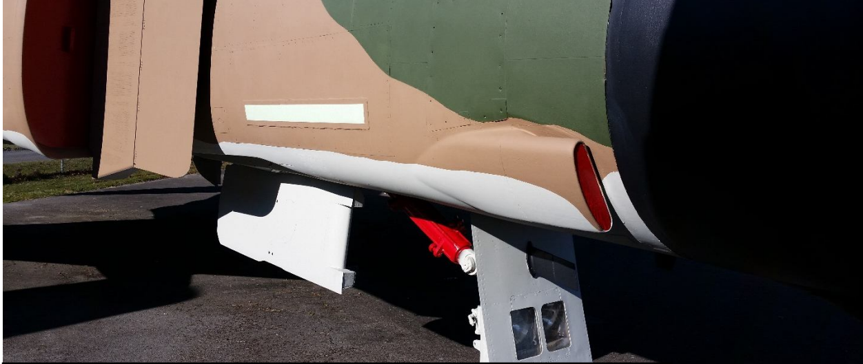
Detail of front section. The small air inlets were used for radar cooling.
