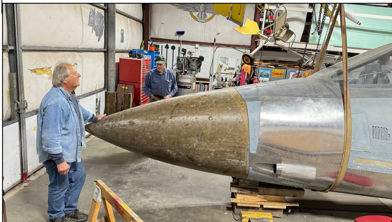
Above: Volunteer Joe Gorman works on ESAM's F-14 fuselage. Below: Fonz DiBlasio (far left) and Peter Bergendahl (back left) admire their work in attaching the radome to the fuselage
