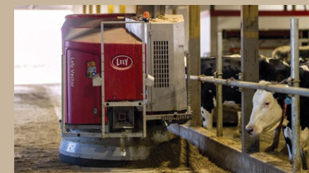
Once mixed, the feeder robots circle the barn, dropping feed along the perimeter.
