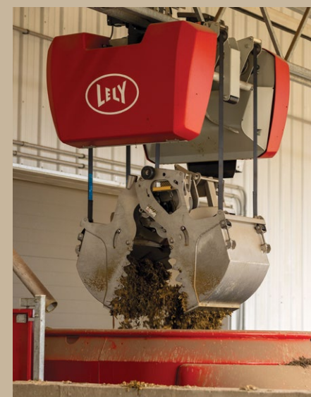
A robotic system grabs hay and corn silage to be mixed within a feeder robot.
